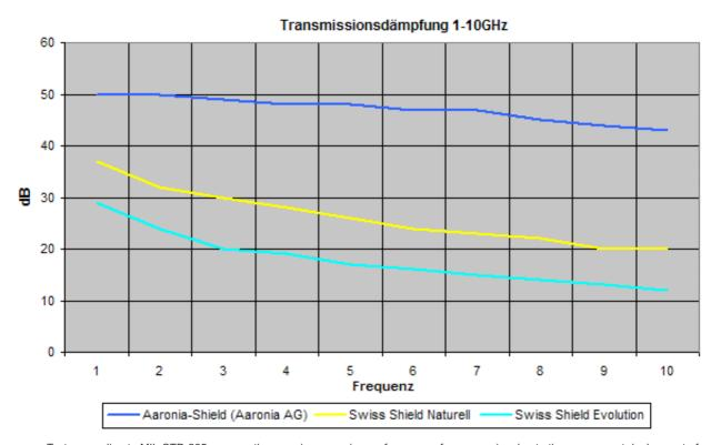
Tests according to MIL-STD-285 approve the superior screening performance of our canopies due to the consequent deployment of Aaronia-Shield®. The RF (high-frequency) radiation damping performance, especially in the frequency range where pulsed signals from cell towers etc. are present, is an exceptional 43dB (99,992%) to 50dB (99,999%). Compared to canopies made from the other products shown, canopies made from Aaronia-Shield® offer 30 to 1000 times better protection!
